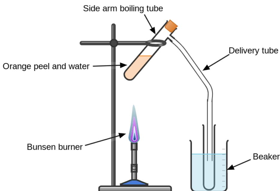
**Figure 1 Experiment Setup**
